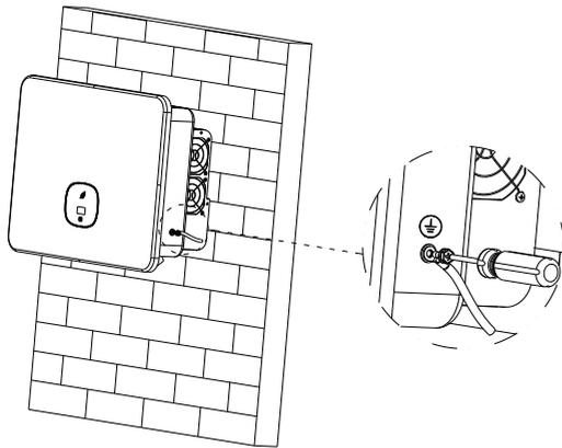
Fig 6.1 Grounding diagram
