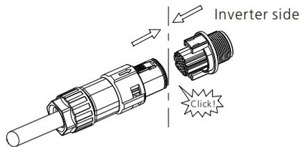
3.Connect the client to the inverter plug until both are tightly locked on the inverter.
