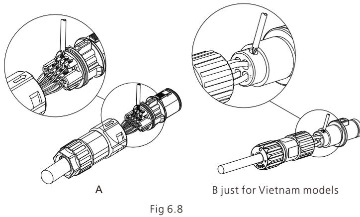
2.Push the threaded sleeve into the socket and tighten the waterproof gland.
