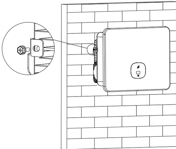
Fig 5.9 Schematic diagram of inverter wall mounting
