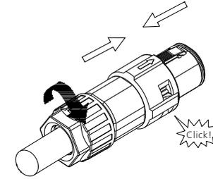
Remove the signal connector
