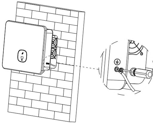
Fig 6.1 Grounding diagram
