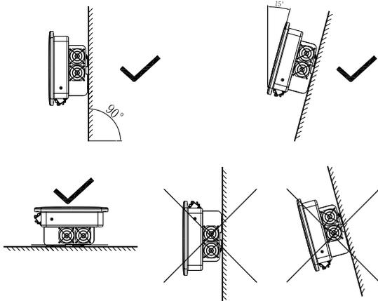
Fig 5.1 Installation diagram
