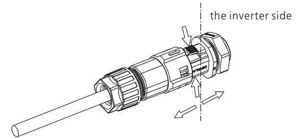
2. Insert the H-shaped tool and pull it out of the socket.
