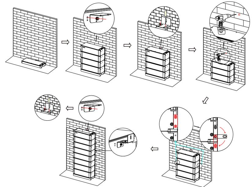
Fig 4.8: Floor standing installation process
