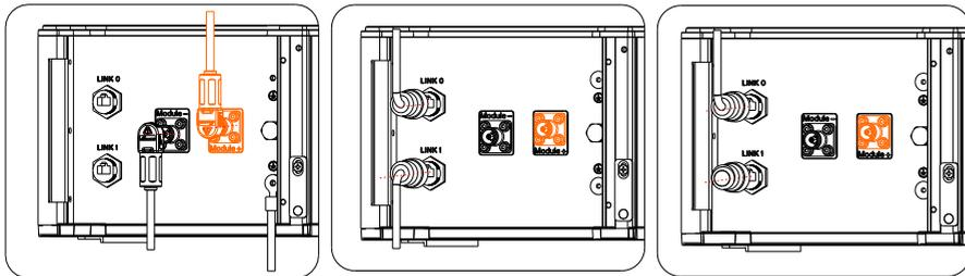
Fig 4.12: ARK 2.5H-A1 Electrical wiring connection diagram
